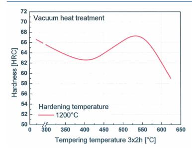
Holding time 3 x 2 hours Specimen size: square 25 mm
