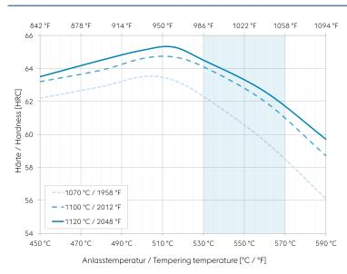
Slow heating to tempering temperature immediately after hardening.
