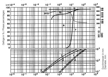
LK... Ledeburitic carbides RA... Retained austenite M... Martensite P... Perlite
