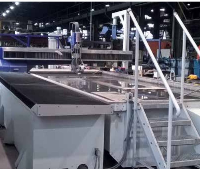
Water jet cutting unit
