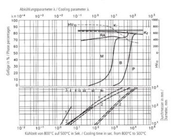
A....Austenite B....Bainite K....Carbide P....Perlite M....Martensite RA...Retained Austenite
